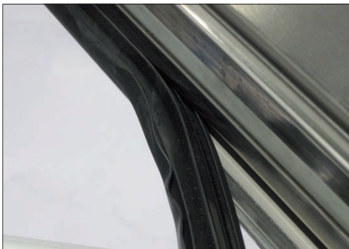
Fig. 287 Inserting the glazing weatherstrip
