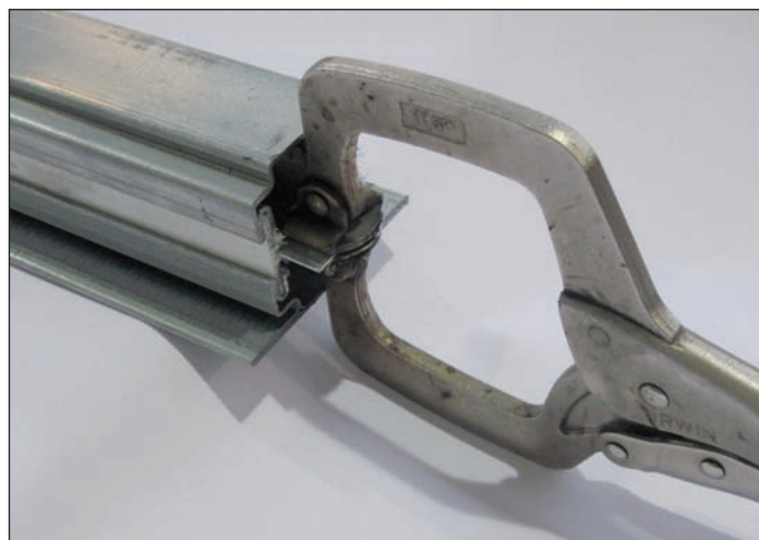
Fig. 23 Alternative: fix the aluminium cover plate in place using clamps
