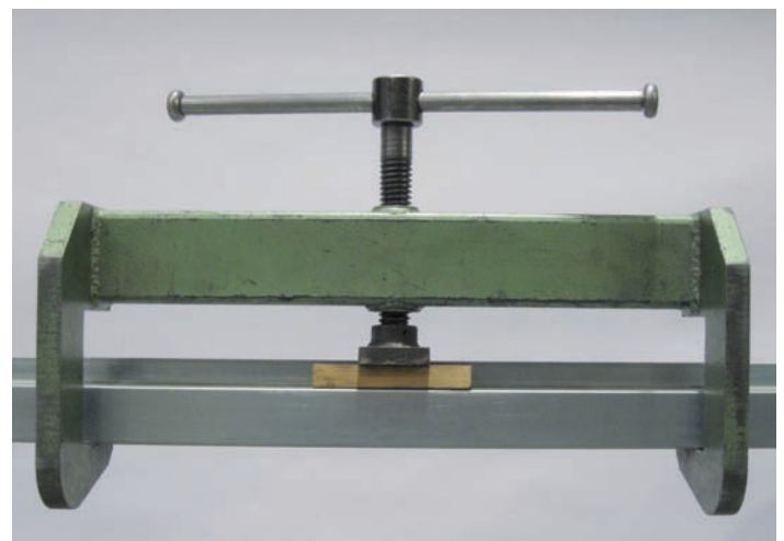
Fig. 123 Aligning tool on the profile
