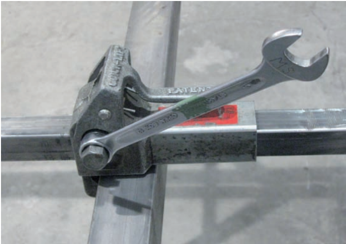
Fig. 114 Aligning tool on the profile
