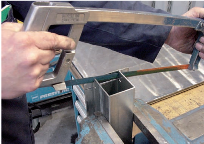
Fig. 41 Cutting using a hand saw (Jansen-Economy and Janisol)
