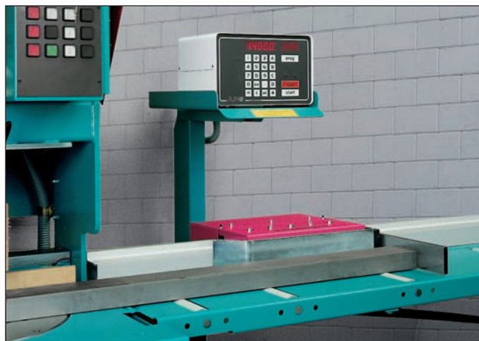
Fig. 13.2 Digital end stop with programming function, automatic action
