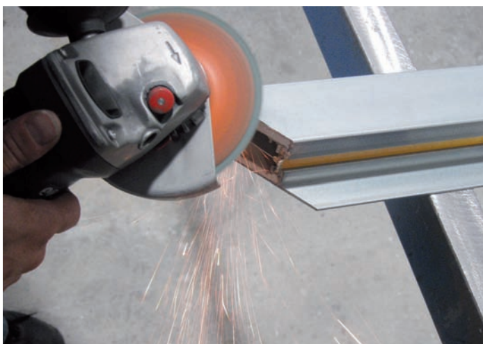
Fig. 69 Chamfer the welded edges at an angle of 45°
