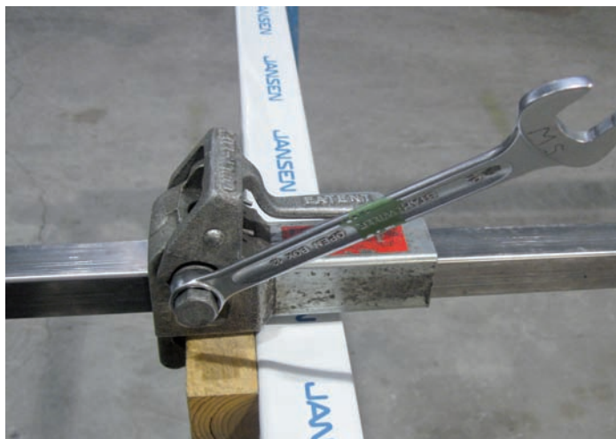
Fig. 186 Aligning tool on the profile (important to use wooden supports for protection)
