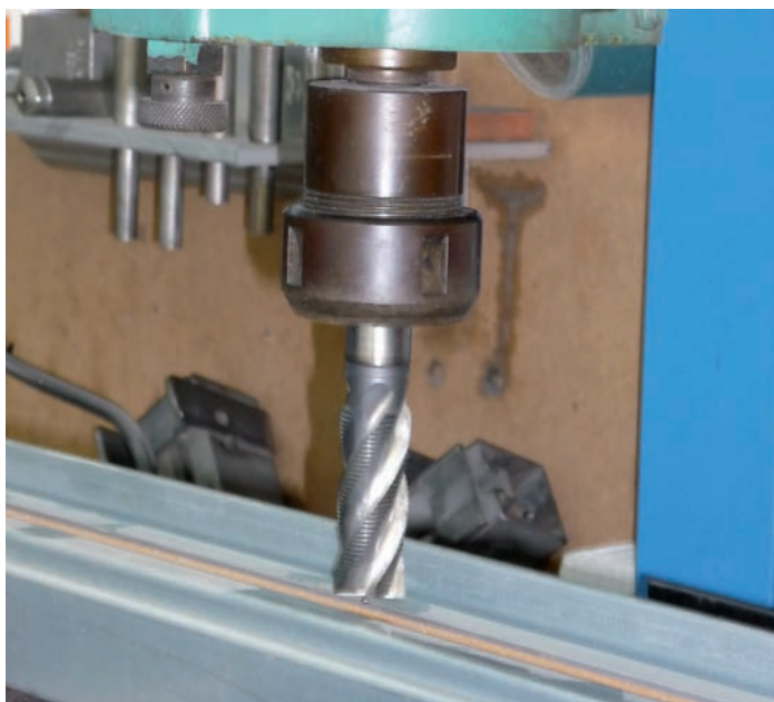
Fig. 50 HSS-PM roughing cutter (TiAlN coating)
