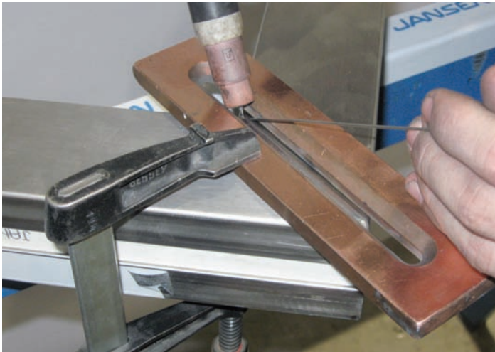
Fig. 173 Stainless steel corner welded with additional wire (build-up welding)
