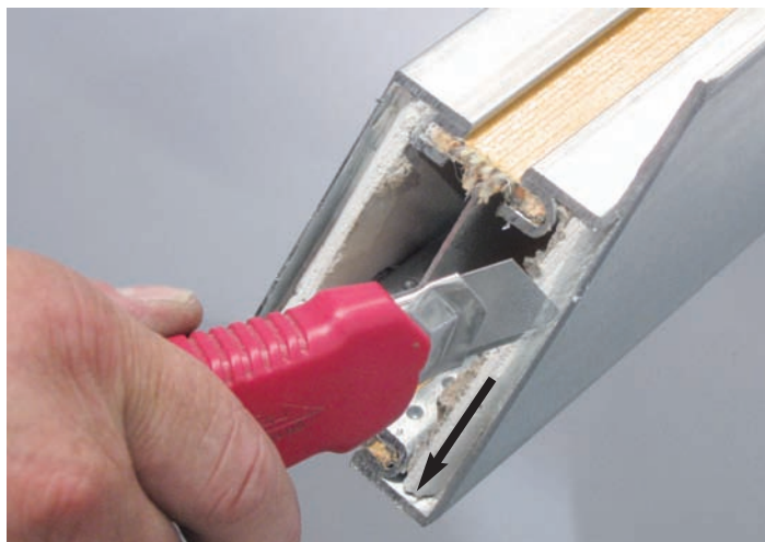
Fig. 70 Freeing the weld seam of Janisol 2 fire protection profiles using a knife
