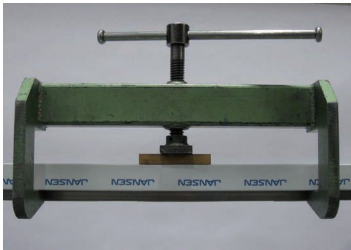
Fig 197 Aligning tool on the profile (important to use wooden supports for protection)
