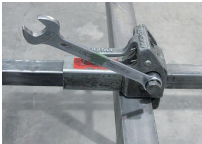
Fig. 112 Aligning tool on the profile
