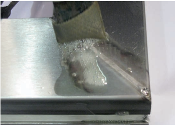
Fig. 201 Pickling the weld seam
