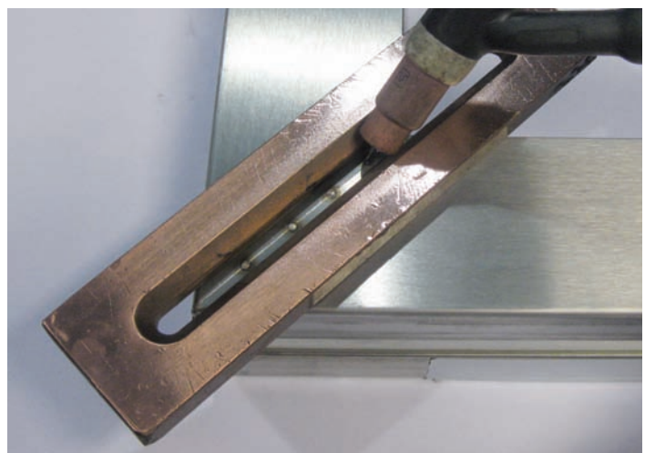
Fig. 159 Copper welding gauge as a welding torch guide
