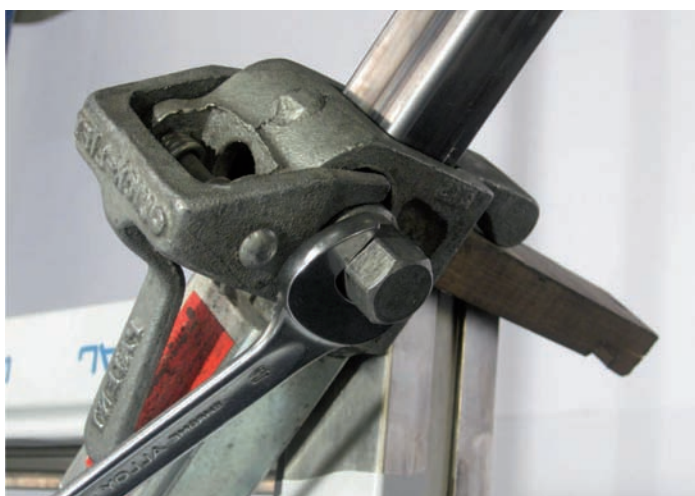
Fig. 189 Aligning tool on the profile (important to use wooden supports for protection)
