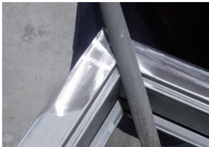
Fig. 136 After fine linishing, file the corners
