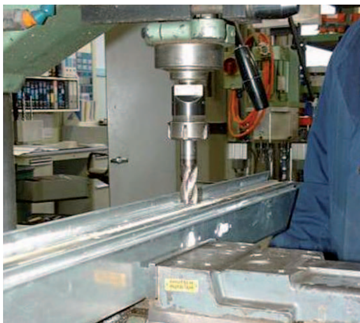
Fig. 49 Lock case longitudinal slot with routing tool
