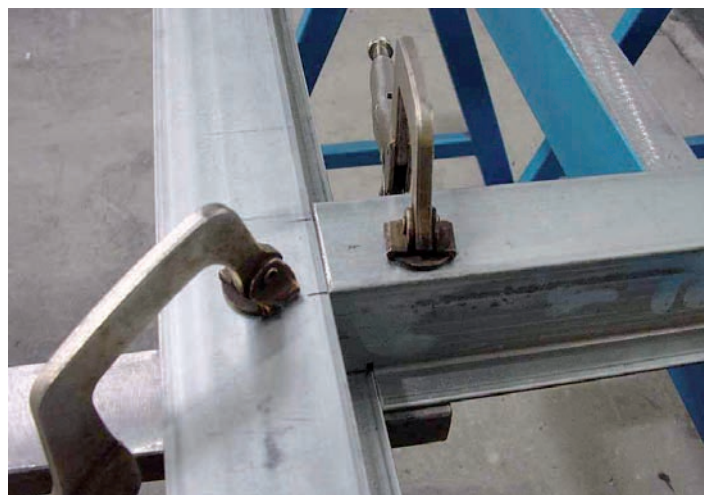
Fig. 75 Clamp mid-rails and transoms using rectangular tube sections and clamps
