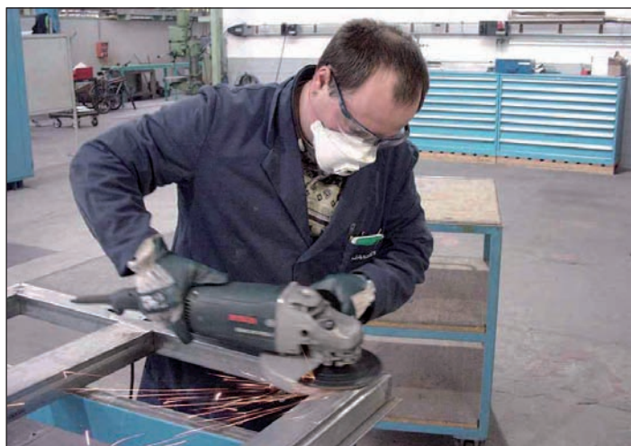
Fig. 210 Machine the welded corner from inside to outside
