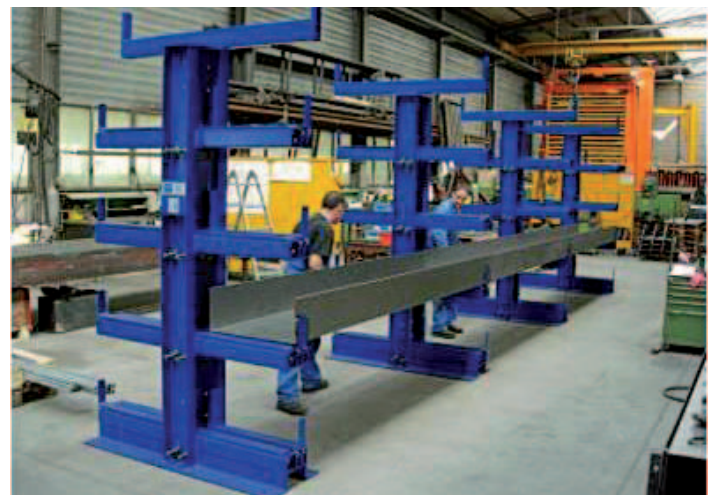
Fig. 12 Option with sheet metal channel for short material
