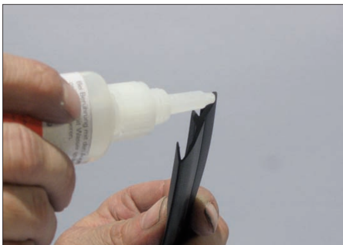
Fig. 288 Bonding the corner
