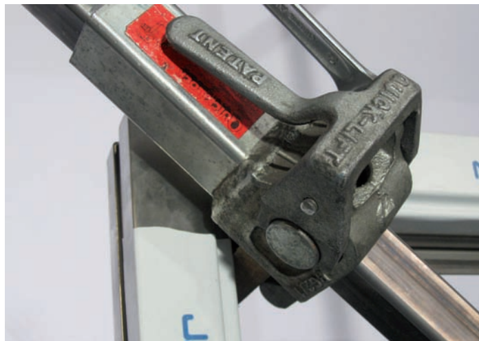
Fig. 191 Aligning tool on the profile (important to use wooden supports for protection)
