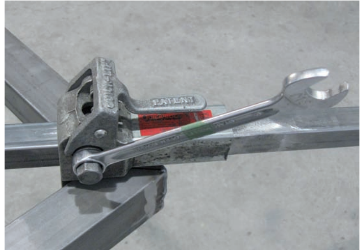
Fig. 119 Aligning tool on the profile
