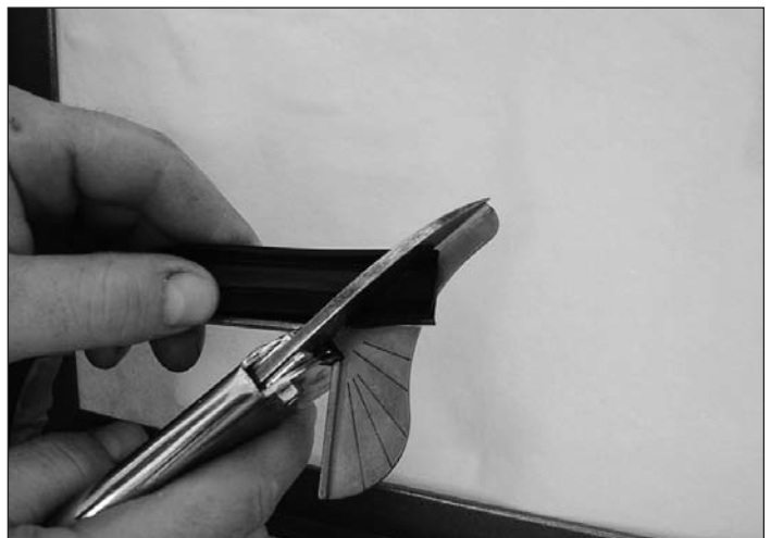
Fig. 275 Cutting the external glazing weatherstrip
