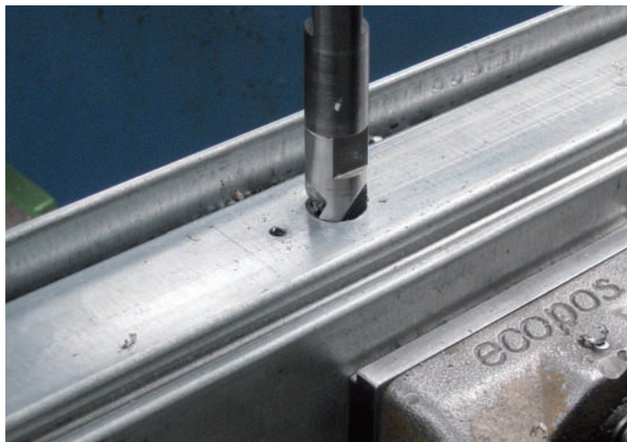
Fig. 47 Drill the lock case end points
