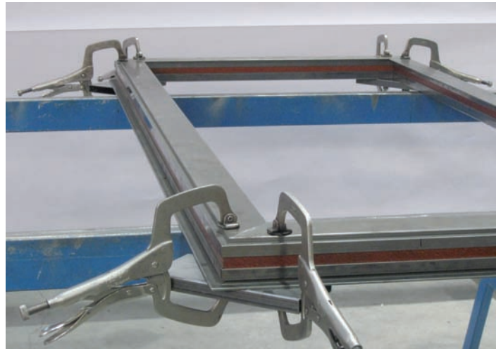
Fig. 73 Clamp the frame constructions using quick action clamps
