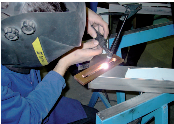
Fig. 175 Stainless steel corner welded without additional wire (fusion welding)
