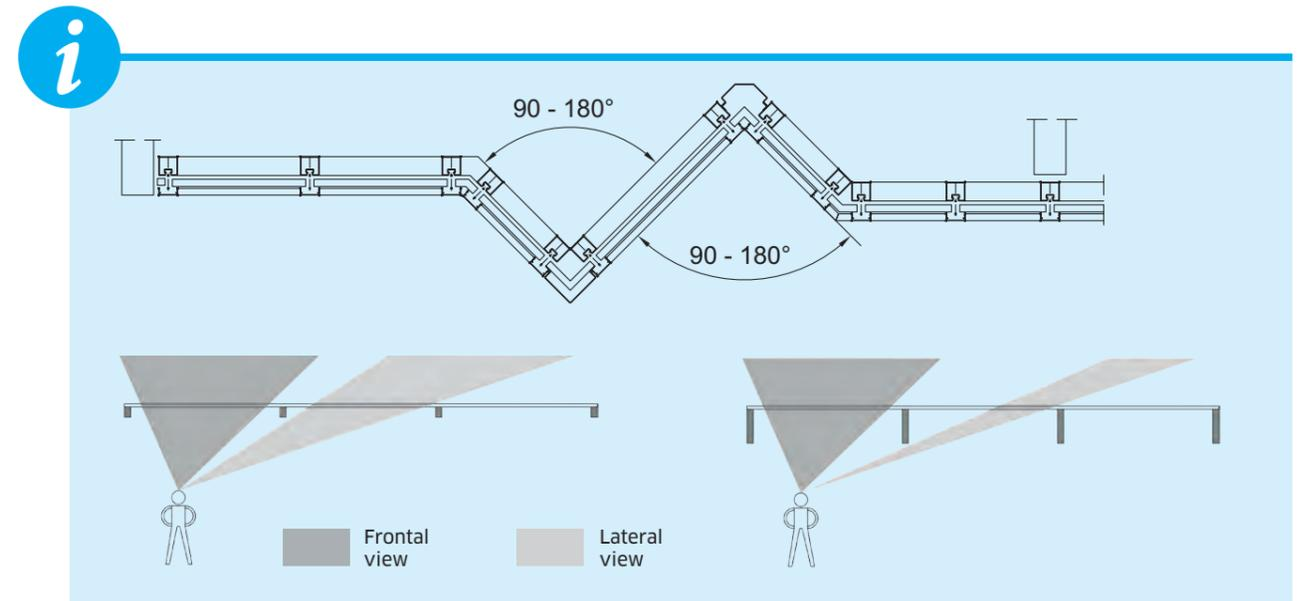
The arrangement of mullion/transom profiles or the view as an SG façade can give very different impressions to the observer.
