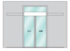
Janisol 2 EI30 fire-resistant sliding doors with "Break-Out" emergency exit function (selection)
