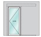
Janisol 2 EI30 fire-resistant sliding doors with "Break-In" emergency exit function (selection)
